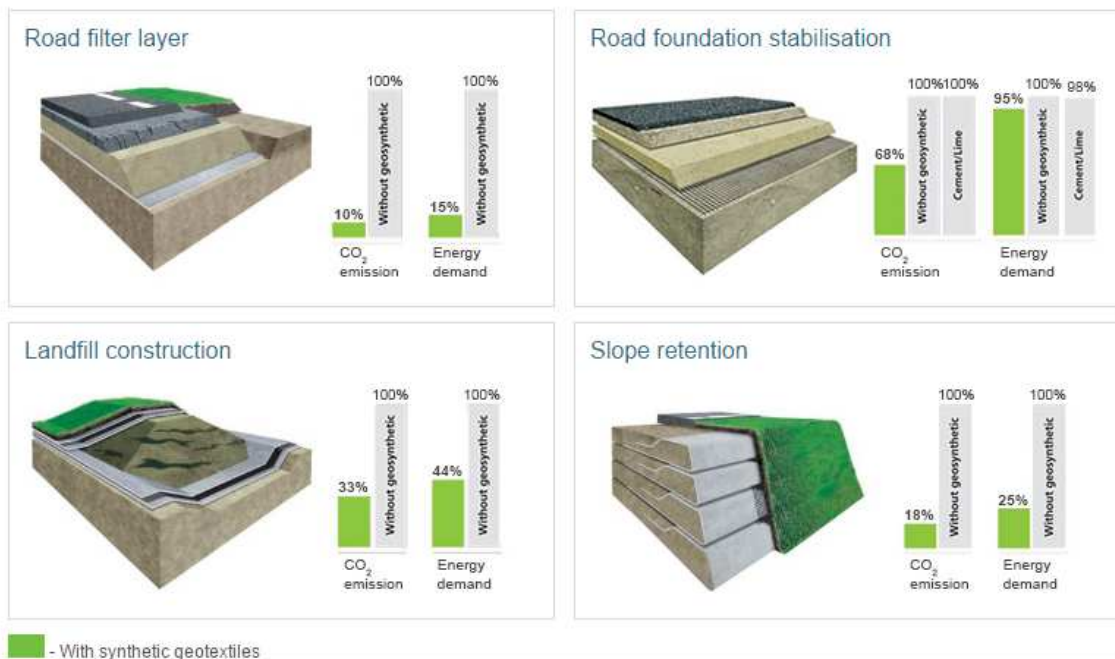
Figure 7. Summary of savings in CO 2 emissions and energy intensity structures in % with and without the use of geosynthetics.
